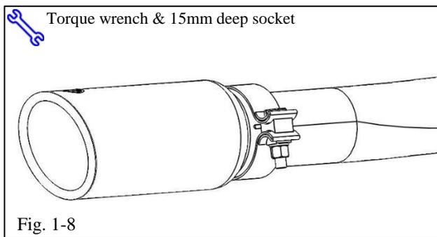
**STOP** (h) Torque clamp nut to 55 N-m (41 ft-lbf) (Fig. 1-8).
