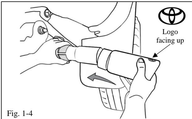
(e) Slide the exhaust tip over the tail pipe with the logo up (Fig. 1-4 & Fig. 1-5).
