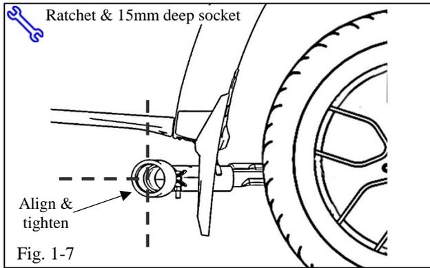
(g) Once the tip is positioned correctly and the alignment seems accurate, tighten the clamp nut making sure the bolt remains in a vertical 3 o'clock position (Fig.1-7).
