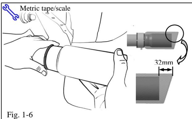
**!** (f) Continue sliding the exhaust tip over the tail pipe for an approximately 32mm distance between the end of the tail pipe and the end of the exhaust tip (Fig. 1-6).
